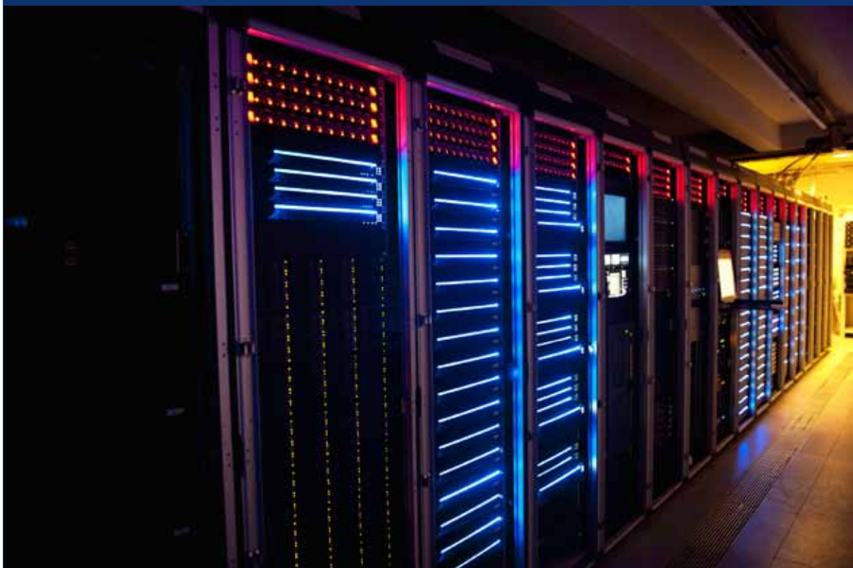
Figure 2.1: Inside a cloud computing data centre, large numbers of individual computers are stacked in racks and any number of them can be remotely accessed via the internet as and when users require them. Typically, users pay only a small rental cost for each hour's access to each computer, so super-computer levels of processing power can be accessed at comparatively low cost.
